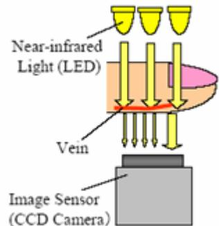
**Figure 2:** Image Acquisition Module
